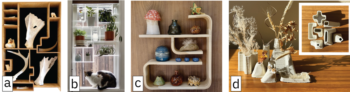
Fig. 1. (a) Uniquely Shaped Spaces generates shelving around personal artifacts. Through three seamful interventions—at maker, machine, and material boundaries—I redirected the system to produce (b) window-fitted shelving negotiating sunlight, plants, and a cat; (c) curved shelving realized through bent lamination; and (d) generated voids realized as ceramic vessels.
